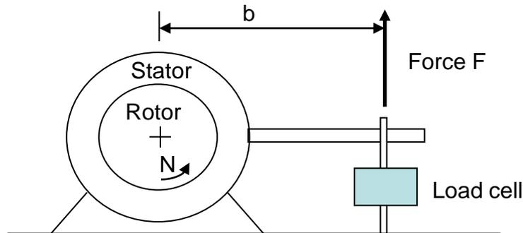
The **torque** exerted by the engine is:  $T = F b$  with units:  $J$
