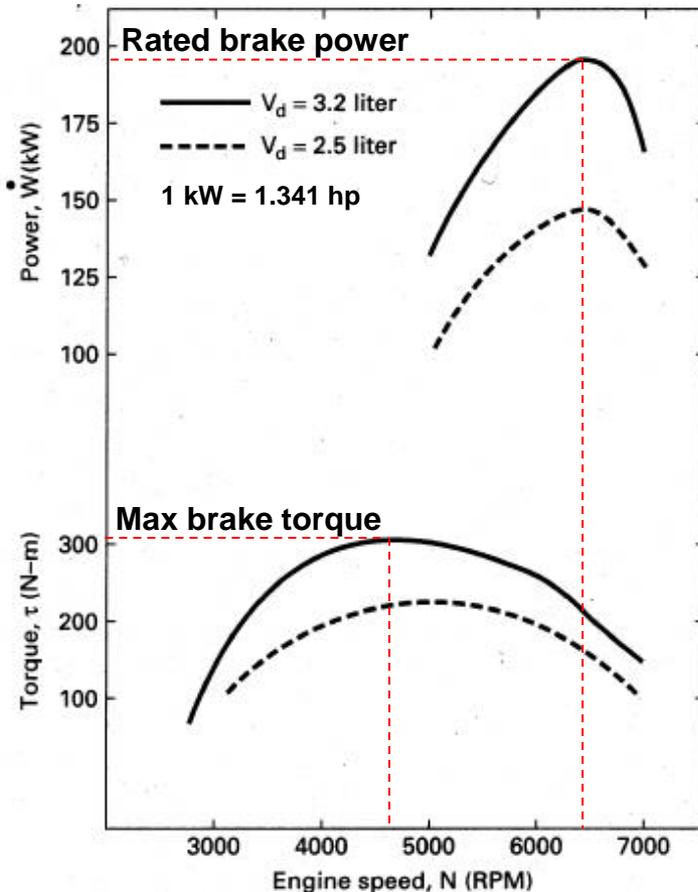
There is a maximum in the brake power versus engine speed called the **rated brake power**.
