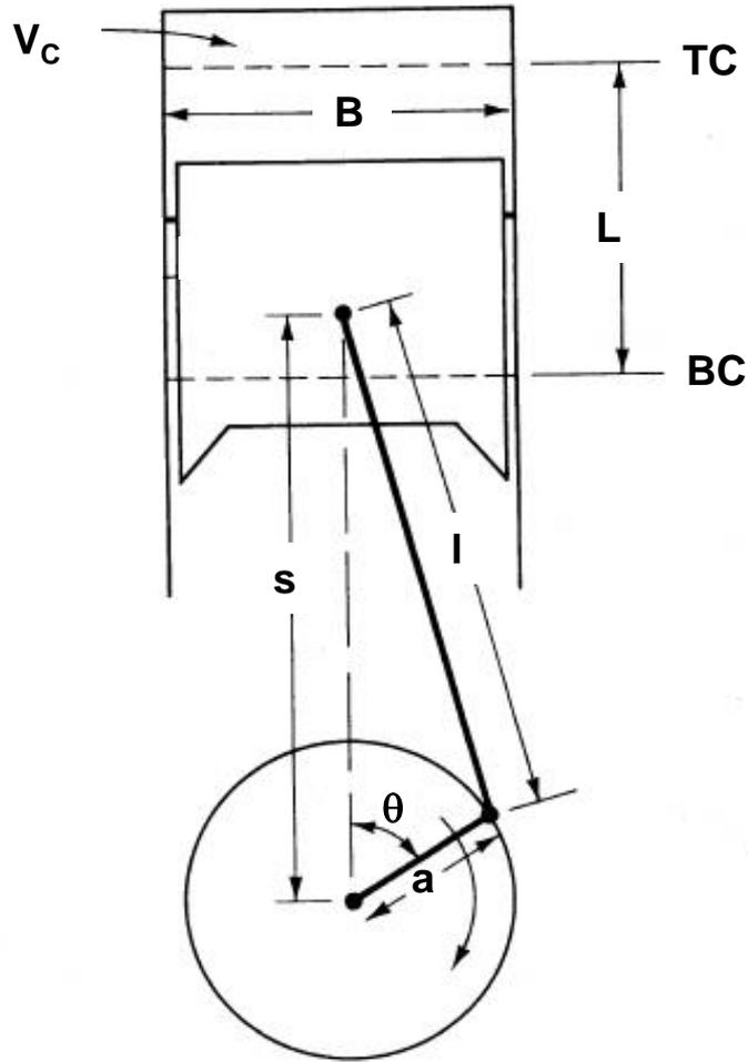
For most engines  $B \sim L$  (square engine)
